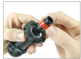
4. Remove the spring, the ratchet and the washer from the freewheel body.
