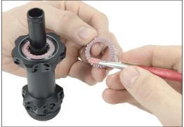
3. Put the spacer onto the axle.
