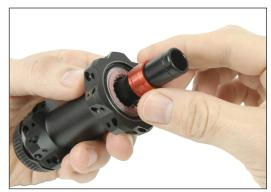
4. Put the spring onto the washer and put the ratchet o to the spring.
