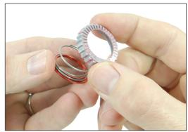
5. Put the washer, spring, and ratchet into the freewheel body.
