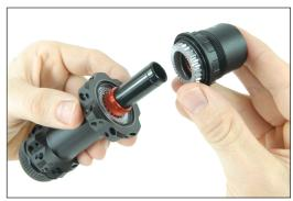
3. Pull the spacer off the axle.
