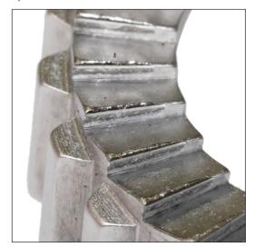
3. Check the internal teeth of the freewheel body for wear.
