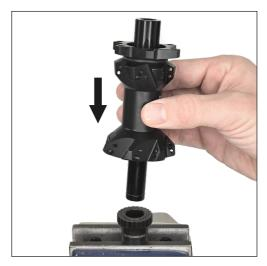
3. Loosen the ring nut by turning the hub counterclockwise.
