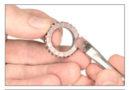
2. Grease the teeth of the freewheel body and the ring nut with DT Swiss special grease.
