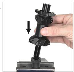
10. Tighten the ring nut as firmly as possible by hand.
